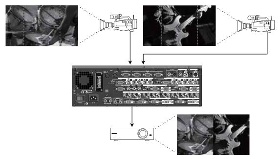
In the split mode, the internal signal flow is as shown below.
