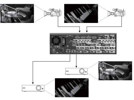
In the dual mode, the internal signal flow is as shown below.
