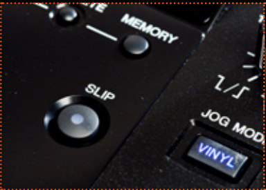
Slip mode allows scratching without affecting track length or losing the beat
